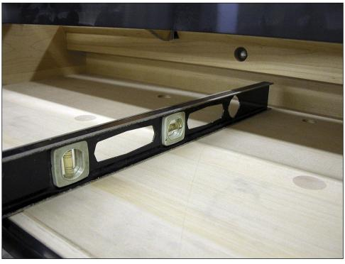
Use a level on the keybed to make sure that the piano is sitting level. It is necessary to level the keybed bass to treble and front to back.
