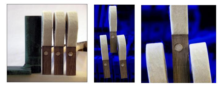
When glued on square, because of hammer front to back movement, clearance will always be a problem. Above you can see what happens when angled hammers are glued on square.
