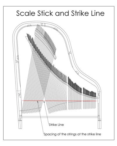
A strike line is a theoretical line that runs across the piano. The intersection between this line and the strings (that is, the center line of the note) defines the point where the hammer hits the string. Sometimes, due to poor execution during the making of the plate, the strike line in actual practice is less then straight. You can be assured, however, that the piano was designed with a straight strike line.
