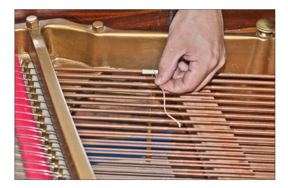
Use the piano technician's plumb bob to transfer the mark on #1 bass string down to the Mylar in the keybed.
