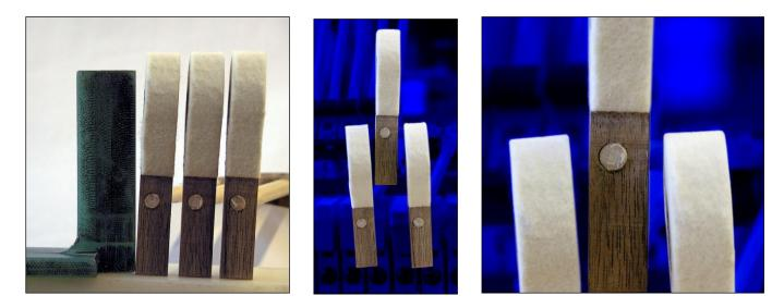
Traditionally, piano makers have tilted the hammers during gluing so as to create clearance. The pictures show clearly how effective the technique is in creating clearance for the hammers.
