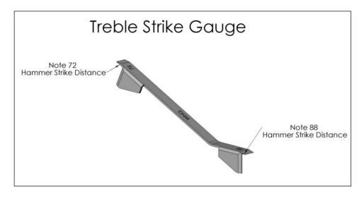
The Treble Strike gauge is a WNG tool that facilitates finding the proper strike point for notes 72 and 88.
