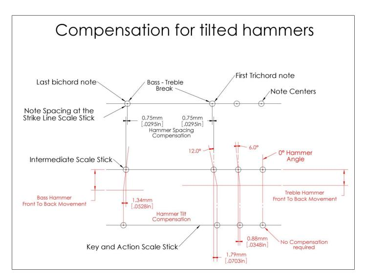
Hammers are bored with angles to match up with the string angles. Because of this, when glued on to shanks, hammers need to be tilted sideways so they will clear the adjacent hammers when played. An alternate method used in Europe is to tilt the travelling instead of the hammer gluing. Either way, the scale stick compensation is the same.
