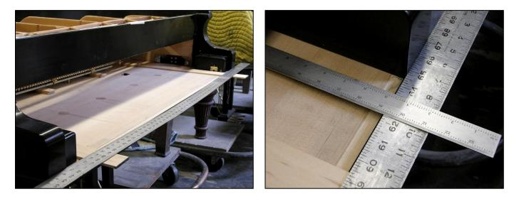
Measure, from the arms of the piano to the strike location at note 88, and mark this on the Mylar at note 1.
