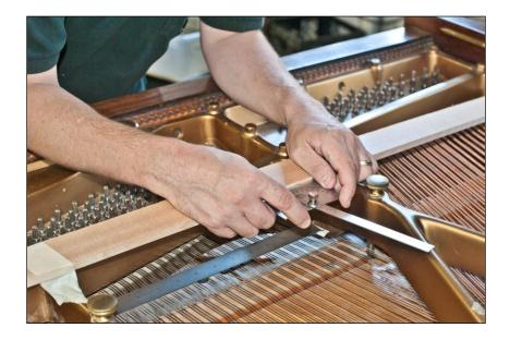
To measure the string angles, you need a straight edge aligned to the strike line to measure from. Place a straight edge on top of the plate bars. Using two small squares align the straight edge to the strike line marks you placed on tape on the strings earlier. Tape the straight edge into place with masking tape so it cannot move while you are measuring the string angles.
