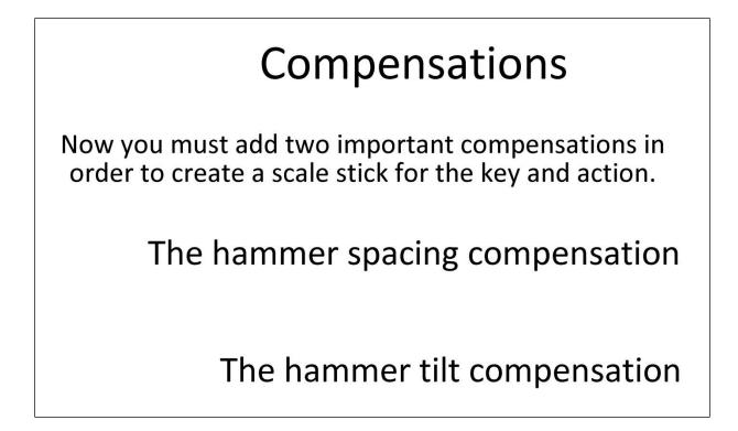
Ideally, after all regulation is complete, the hammer shanks will fall centered above the repetition flange, directly over the cushion. The following compensations are required to meet this criteria.
