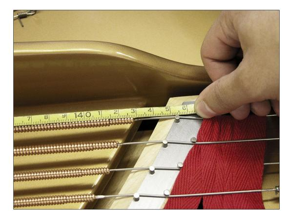
Start by measuring the speaking length for note #1. Use a millimeter tape measure for this task. Since you want to calculate using these numbers, use a measuring device that is decimal to begin with. While you can use fractional English measurements and then convert them to decimal, unneeded work is involved and not very sensible.
