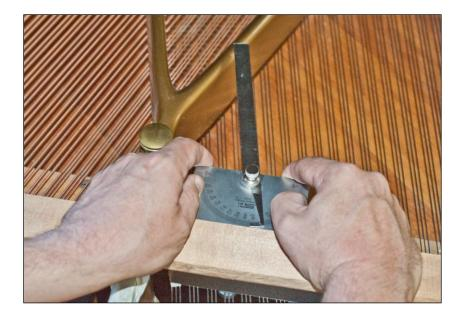
Use a protractor to measure the string angles. Measure as best you can the lowest tenor note to get a sense of the angle. Reset the protractor to nearest whole number angle as close to the angle of the lowest tenor note. For instance we would set the protractor to 12.0° or 13.0° or 14.0° as needed.
