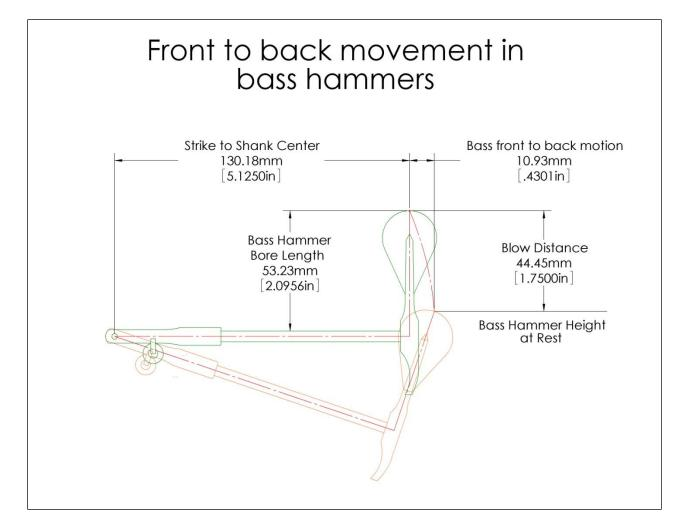
From the above drawings, you see that, as the hammer rotates from its rest position to the string, the tip of the hammer moves forward in the piano.
