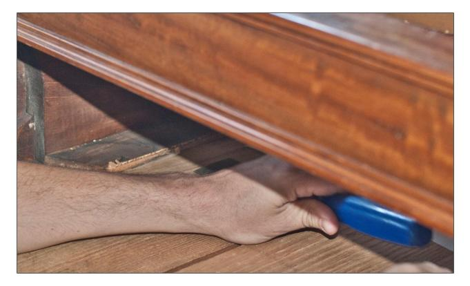
The bass stop block positioned the old action in the piano. Because it will need to be replaced when you replace the keyboard, remove the old stop block as it is in the way and serves no further purpose.
