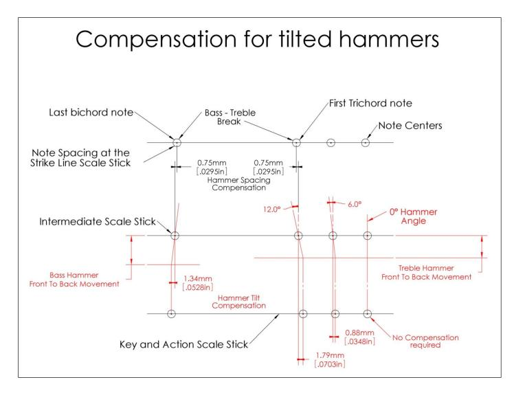
Using the scale stick you created earlier that includes the compensation for soft pedal shift, we will now add the compensation for hammer tilt.
